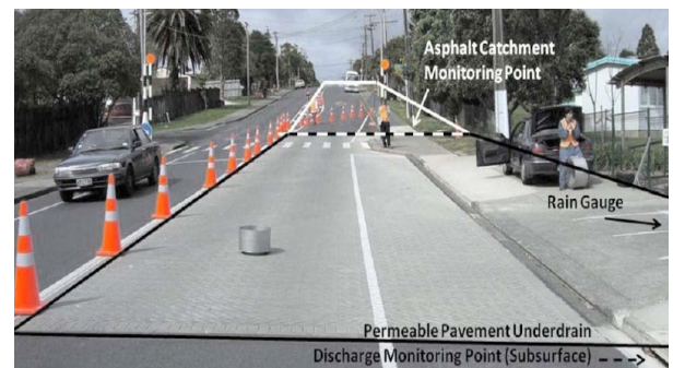
This monitoring site in Auckland, New Zealand tested the effectiveness of permeable pavement on slopes.
